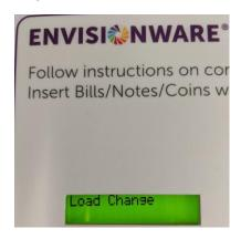
**Step 3.** Press the **RIGHT** button and "Tube:" should indicate "0.00" if you have zero out the tubes properly. Insert coins through the top like a patron would to insure coins are being read.
