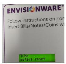
**Step 4.** To exit press the **LEFT** button to get back to "Meters" or press the **RESET** button holding it down for two seconds.
